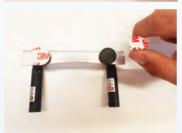
3. Determine the correct position on the generator, remove the strips from the metal discs and stick the unit onto your source.
