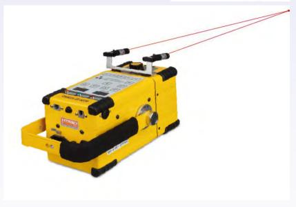
If the laser points don't meet at the cross hairs projected by the collimator light, adjustments can be made.
