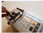
4. Place the Duo Laser Pointer onto the magnetic discs
