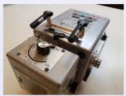
5. Turn on the lasers by pushing the black buttons downwards. Then determine your focal distance and align the lasers to one focal point.
