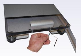
2. Open latch and insert screws bottom-up, then use wrench to screw and tighten grip-handle
